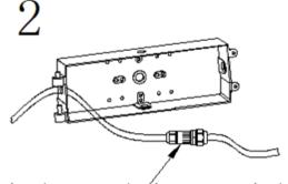
Open the wire-connecting box, connect the input wire of the LED driver with the AC input wire then close the box
