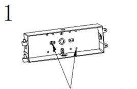
Using screws to install the power supply box onto the solid wall
